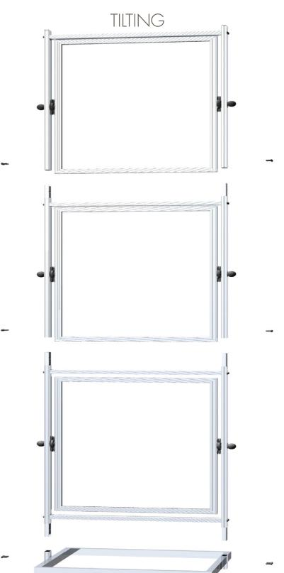
Attach the first frame section onto base using Phillips head screws.
